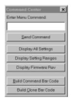
**Build Clone Bar Code** is used to capture the settings from one Imager, and input them to another Imager. When the Build Clone Bar Code button is clicked, Quick\*View captures the settings from the attached Imager and creates an Aztec code which can be printed. (The size of the Aztec code can be altered using the **File - Preferences** selection.) Any Imager that scans the resulting clone bar code will be programmed to the same settings as the original Imager.
